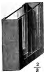
FIG. 76. - Vessel with glass sides for studying the absorption of liquids.
